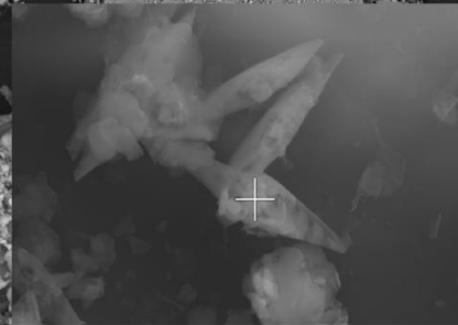
EMPA image (6000x) of bladed precipitates - cross shows location of elemental analysis
