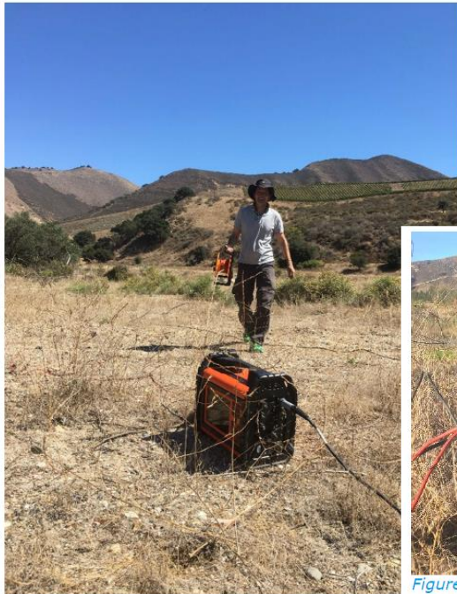
Figure 5 The WalkTEM transmitter cable being positioned.
