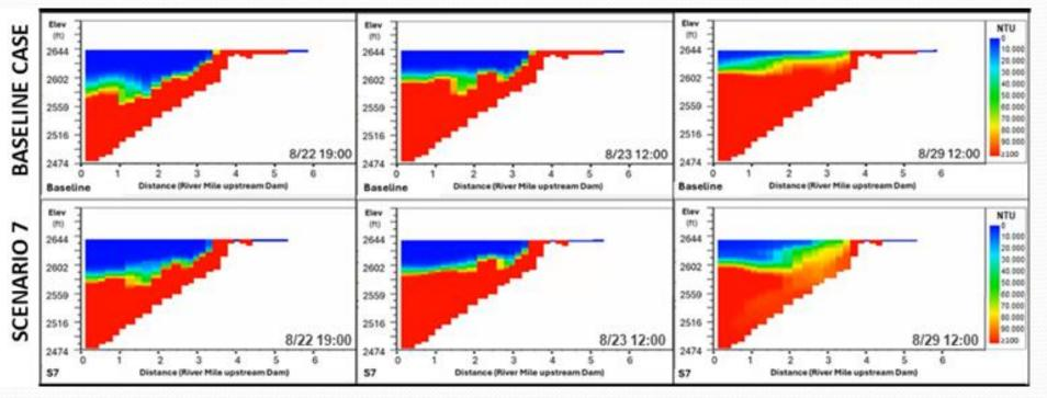
Similar volume where turbidity exceeds 100 NTU due to vertical extent of sediment plume at dam
