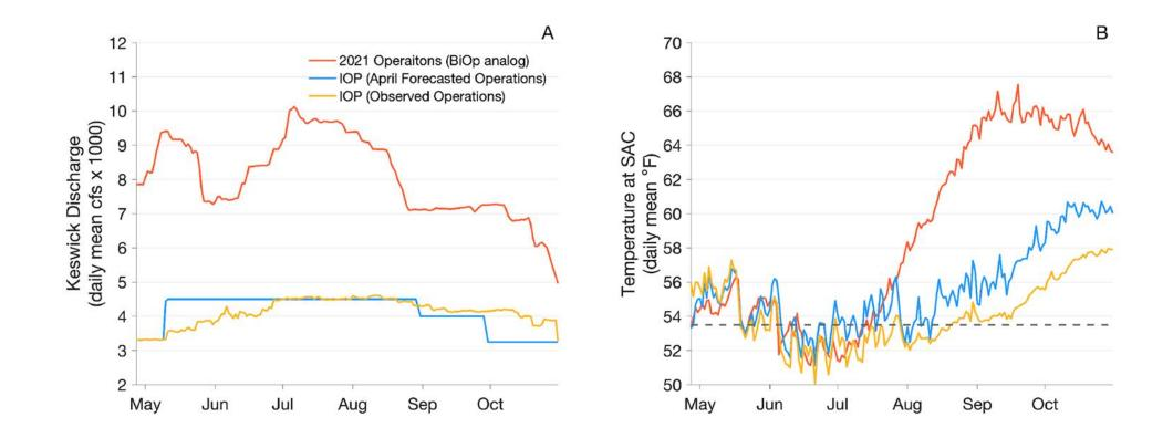
• Time series of Keswick release volume (A) and downstream SAC temperature (B) under the 3 scenarios simulated.
