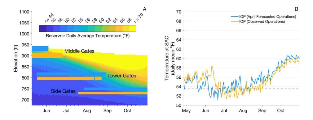
Shasta TCD operations time series (colored horizontal lines) overlaid on Shasta's vertical temperature distribution near the dam (A) and downstream SAC temperature (B).
