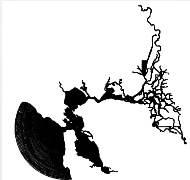
Mesh for Bay-Delta SCHISM
